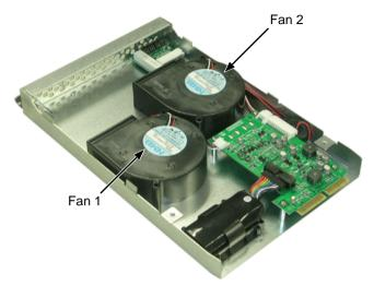
Viewed from the inside (battery) end on the cooling unit, the left blower is Fan 1, the right blower is Fan 2. From the LEDs (see the diagram on page 221), you know which fan to replace.
